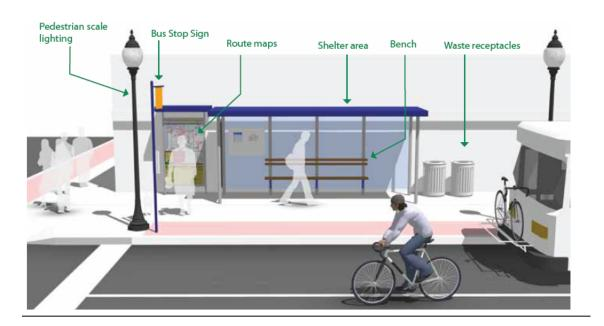
Figure 18: Components of a bus stop
