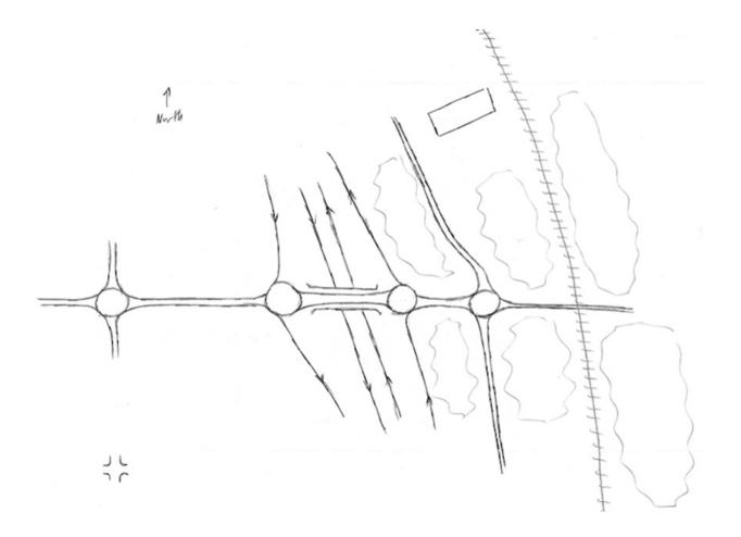
**Concept 3–**A series of roundabouts with an at-grade access to new development:
