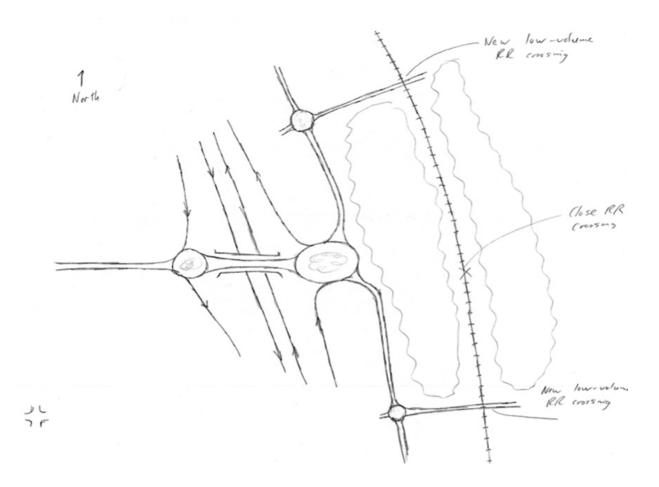
**Concept 4**–A series of roundabouts with a combined ramp terminal/frontage road roundabout:
