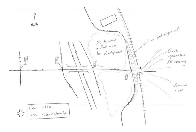
**Concept 2–**A series of signals with grade-separated access to new development:
